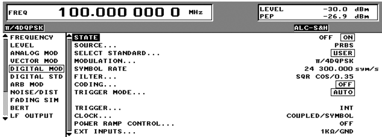
Fig. 2-61 DIGITAL MOD menu, SMIQ equipped with option Modulation Coder SMIQB20 and option Data Generator SMIQB11
